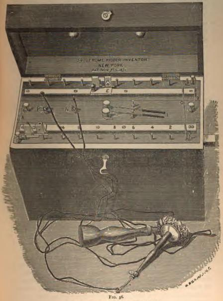
Eighteen-cell zinc-carbon battery (Kidder).
